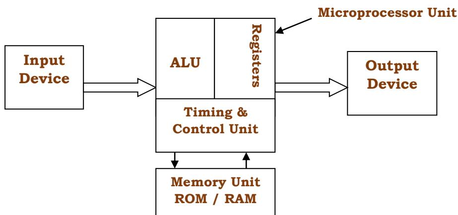
1. Microprocessor is a single chip device which cannot perform any operation alone. It needs some other devices to connect with it for its operation.
