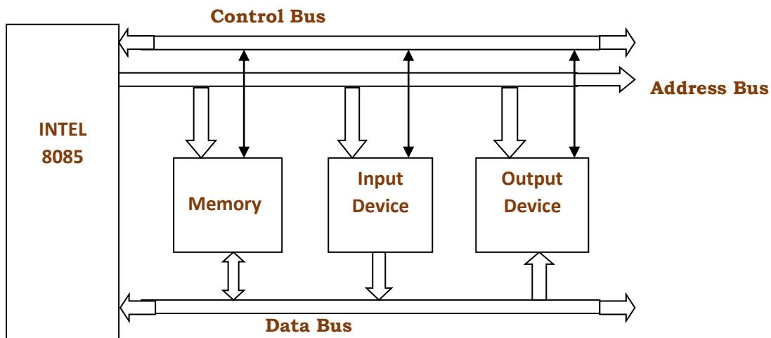
**Address bus** is unidirectional and sends address to all devices outward from the microprocessor. Address for each device is unique to identify the device.
